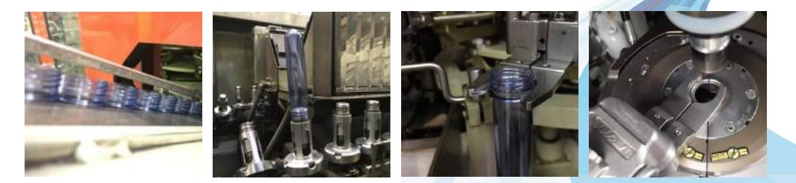
Modification of all machine parts that are concerning loading and insertion of performs Replacing heating oven details necessary to changing diameter or height of the neck finish Pliers and clamping preform details heated by blowing station Modify blowing mould cavity accessory
